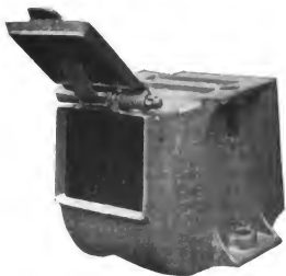
Fig. 4485. Gould Journal Box with Inset Lid and Dust Guard, Type M-P, for Diamond Arch Bar Trucks.
